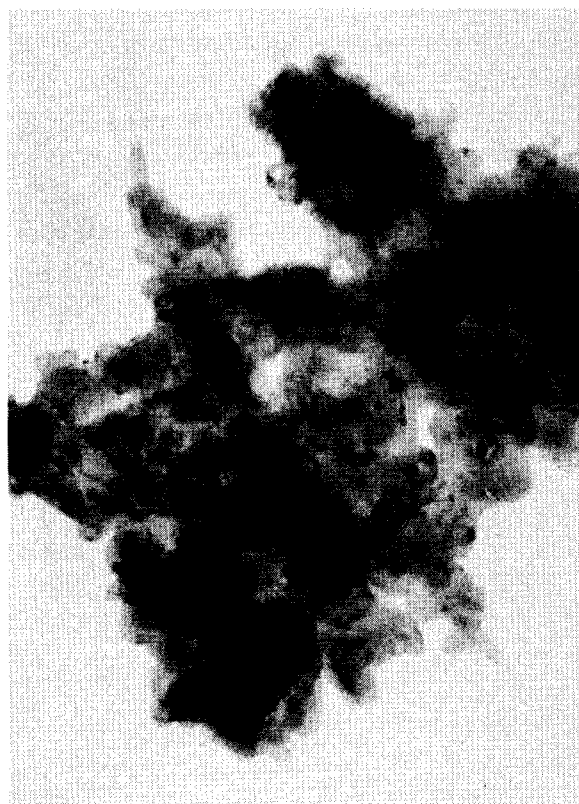
Fig. 6 TEM picture of MgSiO-425 °C sample showing particles of MgO of about 3-5 nm size that are well dispersed on silica surface.
